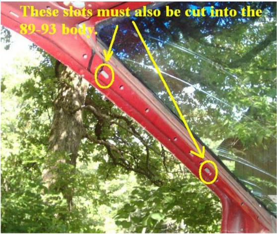
Once the new slots are cut, the A-pillars snap right into place.
