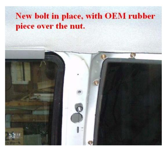
The seat belt retractor mount is already in the correct location. After bolting in the seat belt retractor, install the sail panel, slide the upper seat belt mount over the bolt, and secure it with another nut (once again, using Loctite on the threads of the bolt). Repeat on the other side, and the sail panels are done.
