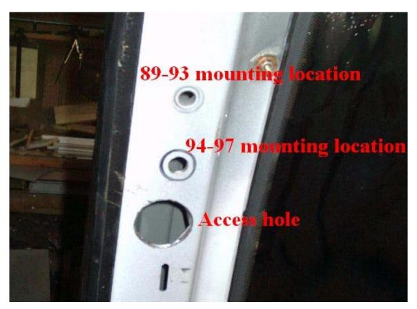
There is a mounting location on the 89-93 body (presumably for the Canadian cars which came with the manual seat belts), however it is approximately 3" higher than the 94-97 location and will not line up with the hole in the 94-97 sail panel.
